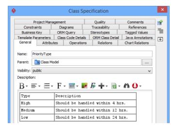
19. You can synchronize the description from class model to the associated entity model by right click on the diagram and select **Utilities > Synchronize Class Description to ERD**.
