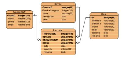
8. Once the entity relationship diagrams are ready, we can then generate class diagrams from our entity relationship model. Select **Tools > Hibernate > Synchronize to Class Diagram** from the toolbar.
